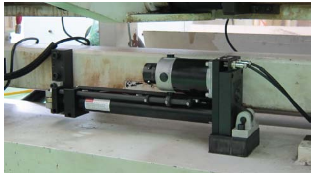
Electrical Actuator SA is used on a Slitting Machine for Unwinding
